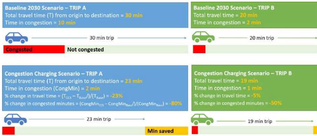
Figure B3-2: Travel time vs. Congested time (Change in minutes and percent change from baseline)
