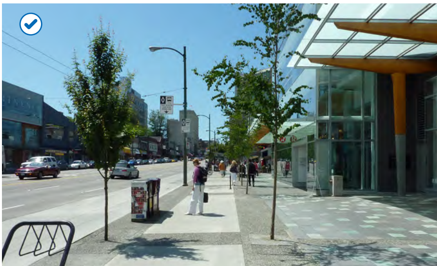
Streetscape adjacent to Broadway–City Hall Station organized to provide good pedestrian comfort, including sidewalk capacity, frontage definition, furnishings and sidewalk edge zones. West Broadway, Vancouver.
